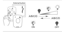
The brightness used last is stored when the unit is switched off. Dimming or switching with one transmitter button (1-button operation).
