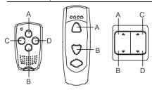
You can change from the operating mode to the programming mode 1 and from one programming mode to the next by briefly (< 1.6 sec.) pressing the programming button: Operating Mode -> Programming Mode 1-> Programming Mode 2-> Operating Mode etc.
